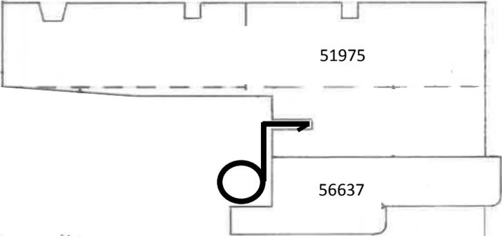
WEATHERSTRIP APPLIED TO HEAD JAMB, SIDE JAMB AND SILL JAMB
