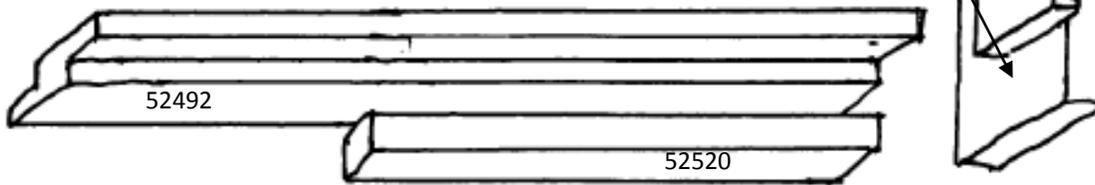
SILL COVER (52492), SIDE AND HEAD COVERS (56637) ARE CONTINUOUS, SILL COVER FILLER (52520) IS NOT, IT BREAKS FOR THE OPERATOR HANDLE
